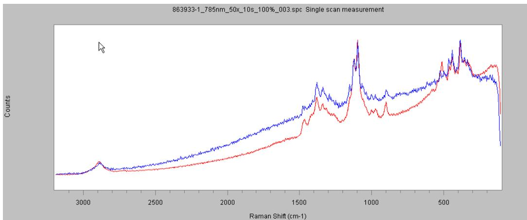
Figure 6: Raman spectrum of sample 863933-1 obtained on cardboard (red graph) and database reference spectrum for cellulose (blue graph).
