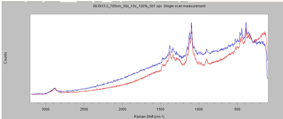
Figure 4: Raman spectrum of sample 863933-2 obtained on sealing (red graph) and database reference spectrum for cellulose (blue graph).
