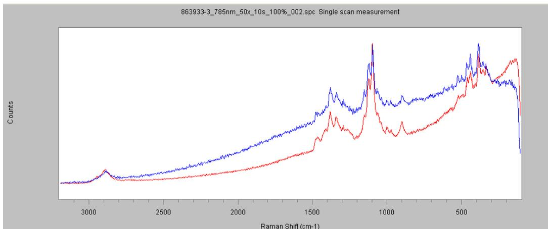
Figure 5: Raman spectrum of sample 863933-3 obtained on tea-bag (red graph) and database reference spectrum for cellulose (blue graph).
