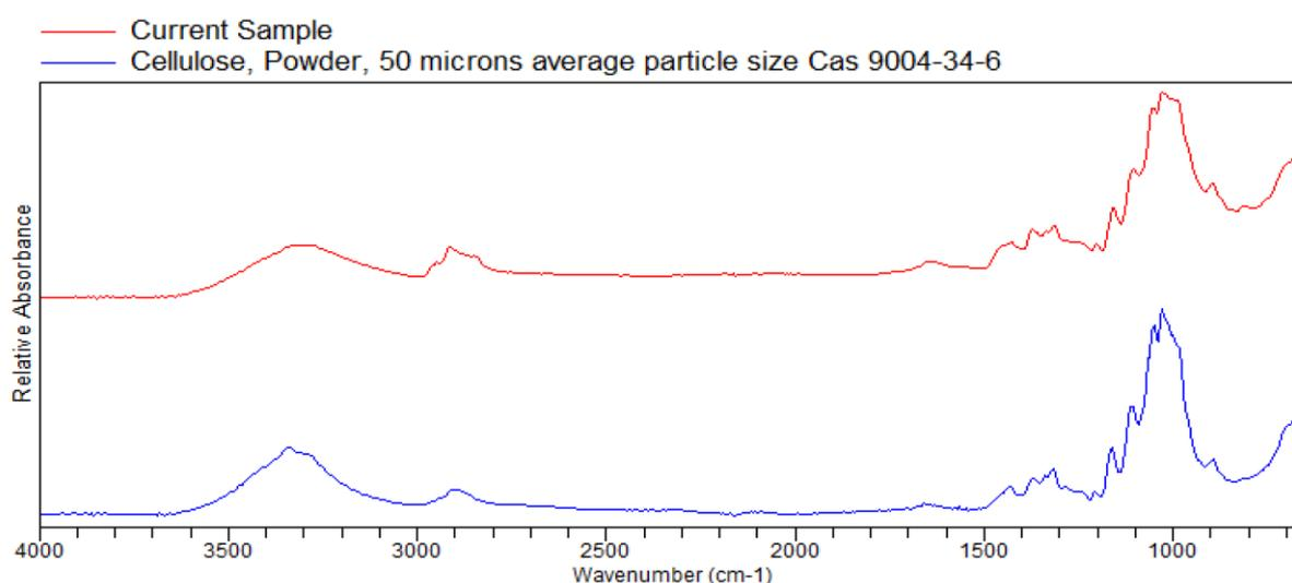
Figure 3: FTIR spectrum of sample 863933-2 obtained on tea-bag (red graph) and database reference spectrum for cellulose (blue graph).
