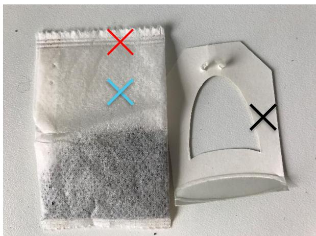
Figure 2: Spots analysed with FTIR and Raman, sealing (red cross), tea-bag (blue cross) and cardboard (black cross).
